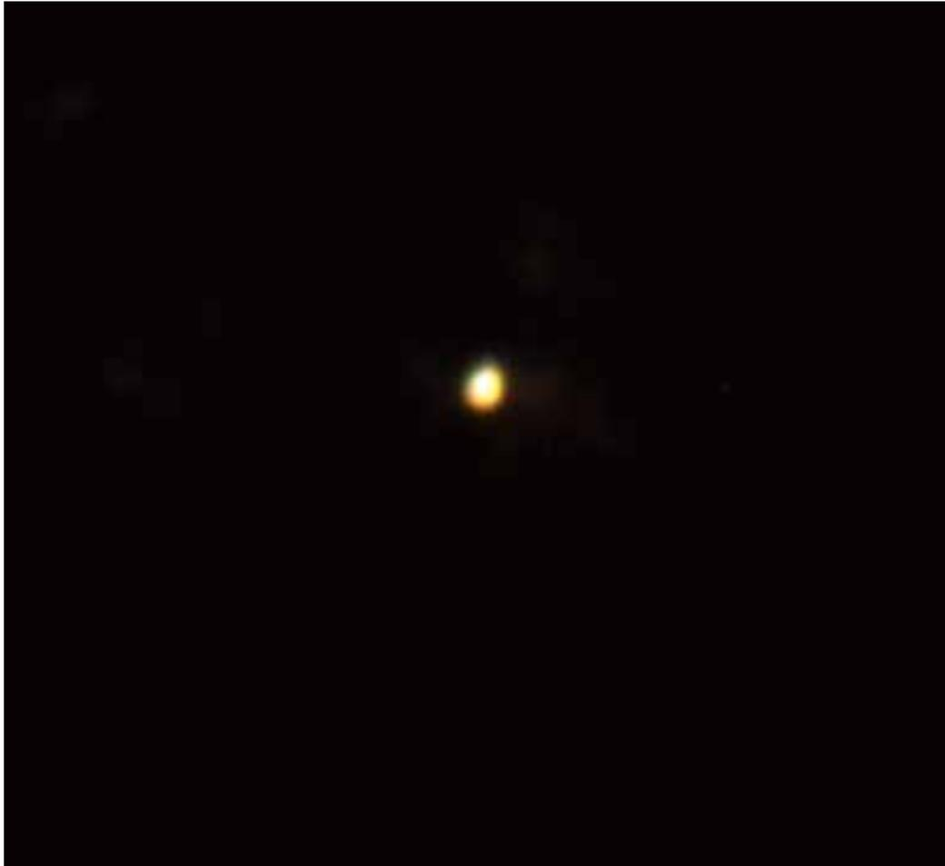
Fig. 1. Optical microscope (back lit) of a barrier where there was a physical hole.
